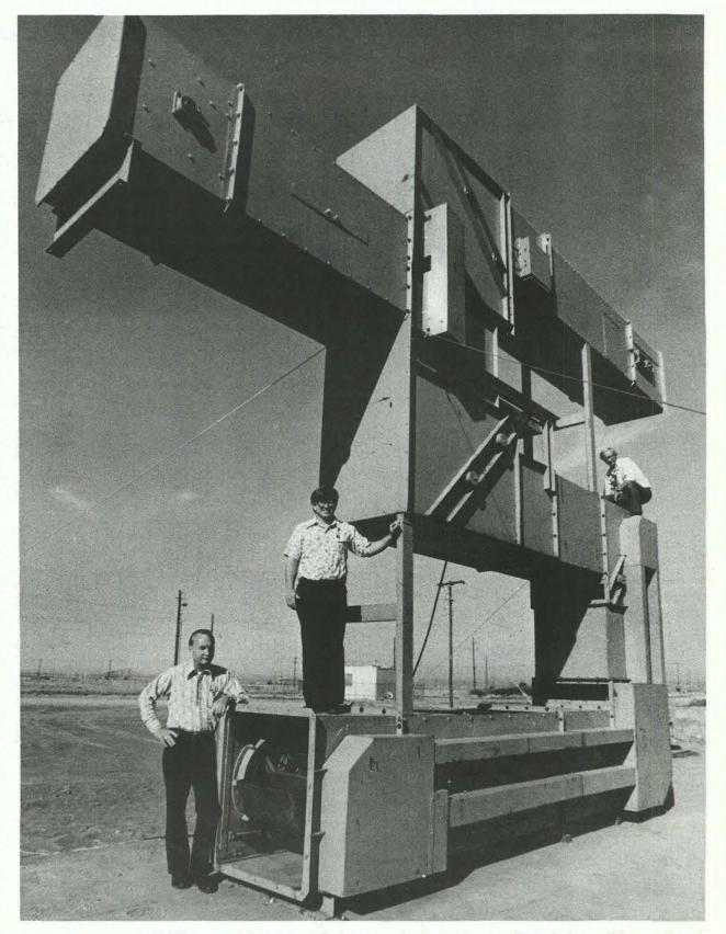
SLUDGE CONVEYOR will be one of the principal elements of pilot facility in which sludge will be irradiated to eliminate pathogens. Aim is to produce material suitable for use as a fertilizer or soil conditioner. From Beneficial Uses Program Division 5445, Jack Sivinski, Marvin Morris and Jim Pierce stand with machine.
